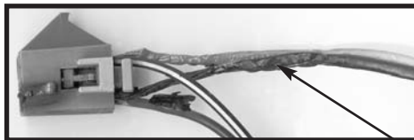
Notice wire insulation is only melted close to connector.
