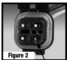
Figure 2 Blackened and/or melted area on harness connector indicates a problem.
