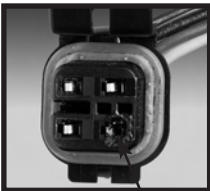
Blackened and/or melted area on harness connector indicates a problem.
